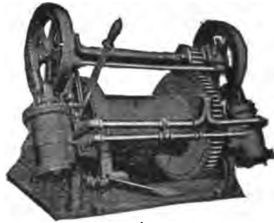
BACON'S Double Cylinder Friction Drum WINZE HOIST For Underground Use in Mines
